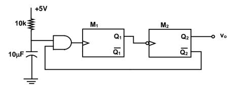
The monoshots  $M_1$  and  $M_2$  when triggered produce pulses of width  $T_1$  and  $T_2$  respectively, where  $T_1 > T_2$ . The steady state output voltage  $v_0$  of the circuit is
